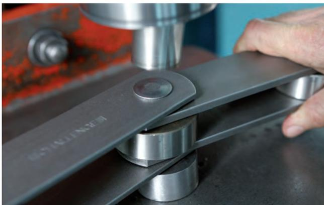
As specialists in the production of spin-riveted chains, we use high-grade case-hardened alloy steel pins produced on state-of-the-art European machines, giving you the best rivet on any standard chain.
