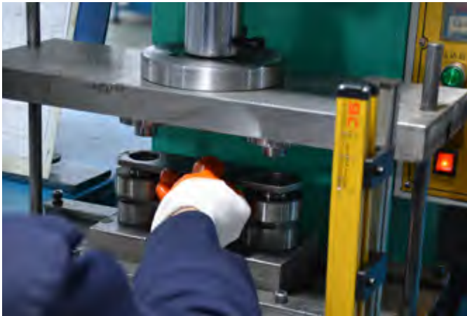
Pins with location shoulders/flats and interference fit Precise positioning of outer plates adds to strength whilst ensuring accuracy of attachment positioning
