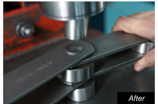
Pins with location shoulders/flats and interference fit Precise positioning of outer plates adds to strength whilst ensuring accuracy of attachment positioning
