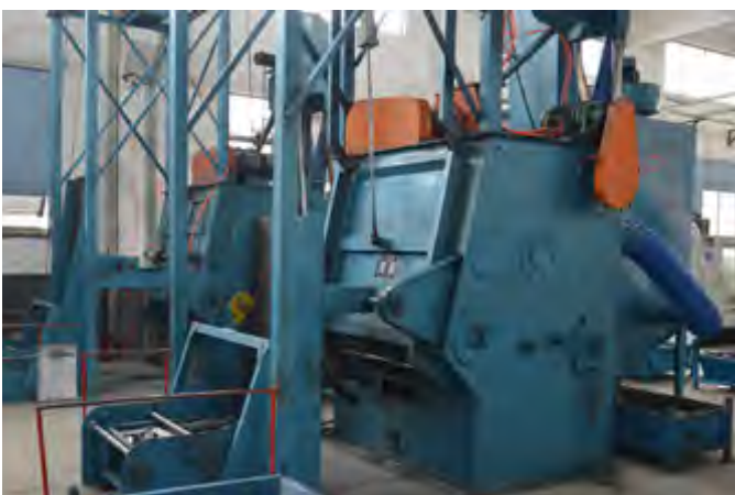
Shot peened to produce a strong surface and reduce fatigue
