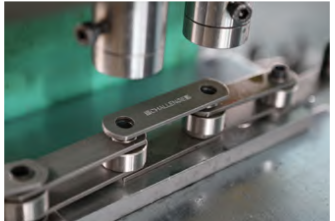
Pins with location shoulders/flats and interference fit Precise positioning of outer plates adds to strength whilst ensuring accuracy of attachment positioning
