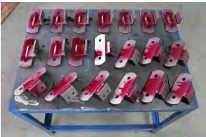
Dye pen testing of welds
